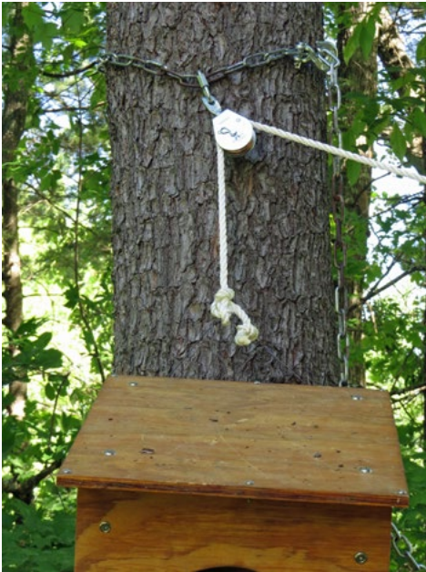
Close-up of chain-pulley-rope mount.
