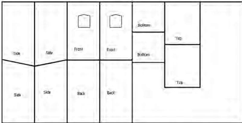
Barred Owl Nest Box Cut Diagram. 4 x 8 pressure treated plywood. Sides, back, front 13 inches wide. Sides 24.25 inches in back, 23.75 inches in front. Bottoms 12 x 13 inches. Tops 14 x 17 inches. Entrance hole is 7 x 7 inches. Bottom of hole is 13 inches above bottom of the front panel. 1.25 inch square balusters in interior corners to screw plywood to.
